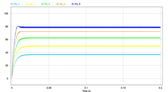
Figure 173 PV power with MPPT for varying irradiance
