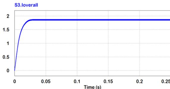
Figure 8 Output current of the converter
