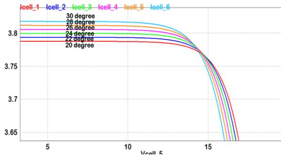
Figure 138 I vs. V with varying temperature
