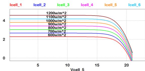
Figure 116 I Vs. V with varying irradiance
