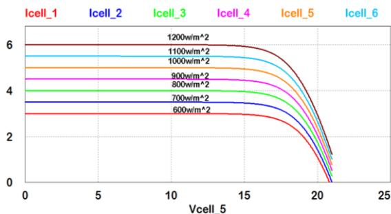
Figure 2 V-I Characteristics of PV
