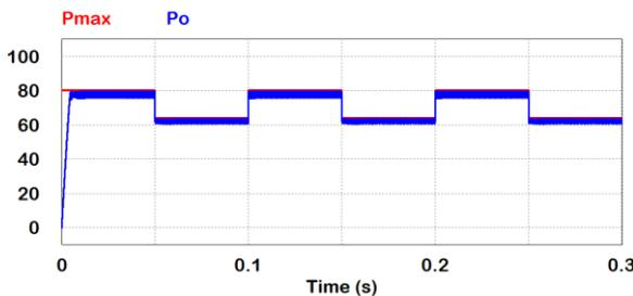
Figure 151 PV power without MPPT
