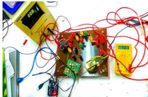
Figure 24 Prototype of the proposed DC-DC Converter
