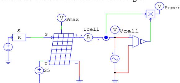
Figure 1 PV Model using PSIM
