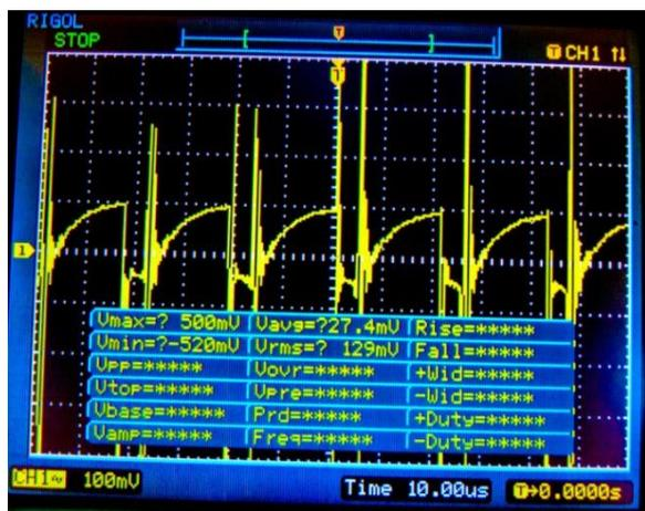
Figure 26 Output voltage ripple of the DC-DC Converter
