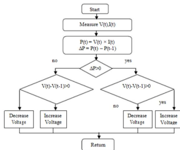
Figure 72 Flow chart of MPPT algorithm
