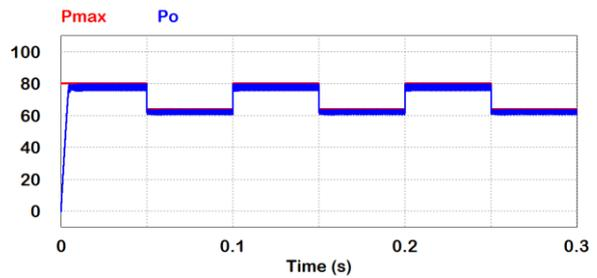
Figure 162 PV power with MPPT
