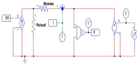
Figure 3 Equivalent circuit of PV
