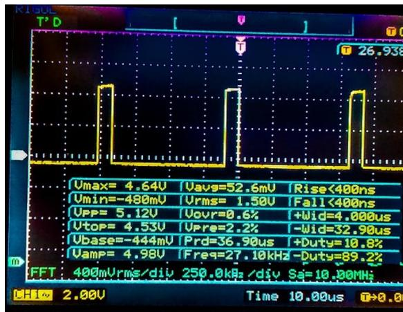
Figure 25 Gating pulse for the proposed DC-DC converter
