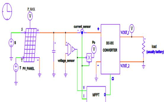
Figure 83 PSIM circuit of superlift converter with PV as source with MPPT
