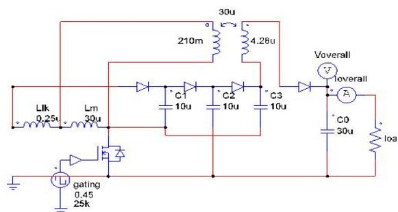
Figure 4- Circuit Diagram of super lift DC-DC converter
