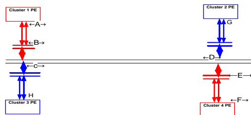
Figure 2 Schematic of a maximum wire span during Processing Elements communication in HSBSM
