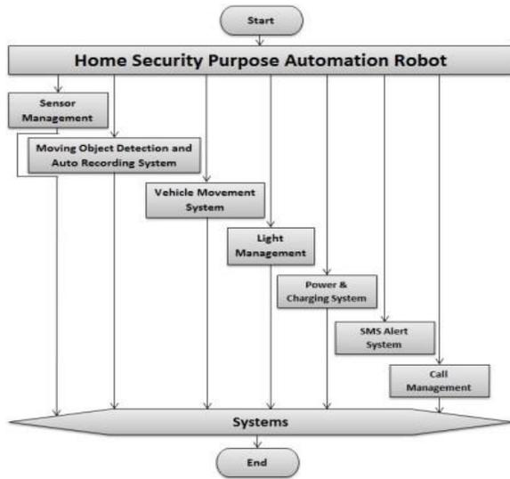
Figure 1: Automation Home Security Robot System Architecture.
