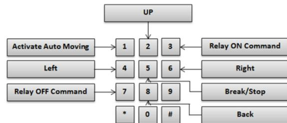
Figure 5: Bluetooth & DTMF Controlling System.
