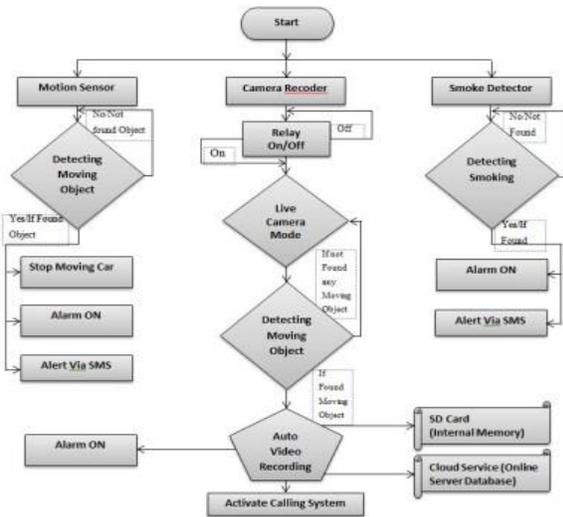
Figure 3: Moving Object Detection and Auto Recording System.
