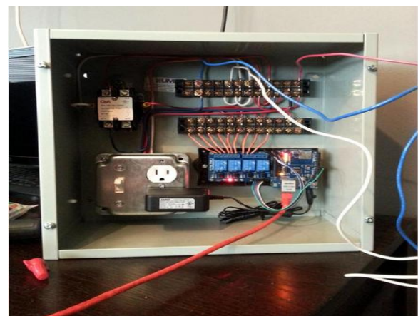
Figure 8 Arduino and modules are inside on Board for implementation.
