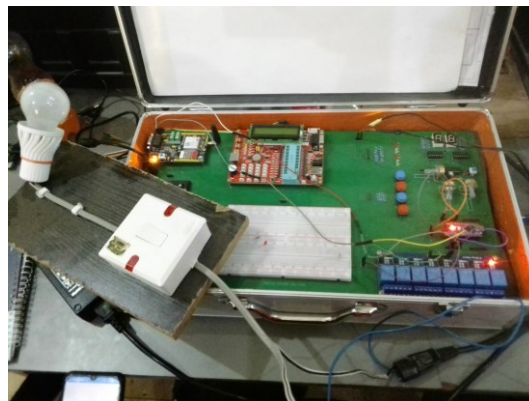
Figure 7 Overall system setup with appliance
