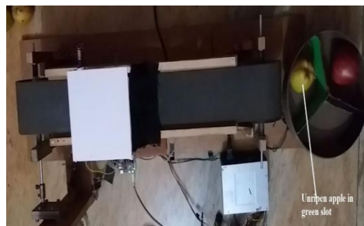
Figure 5.4 Detected unripe apple is collected in green slot.
