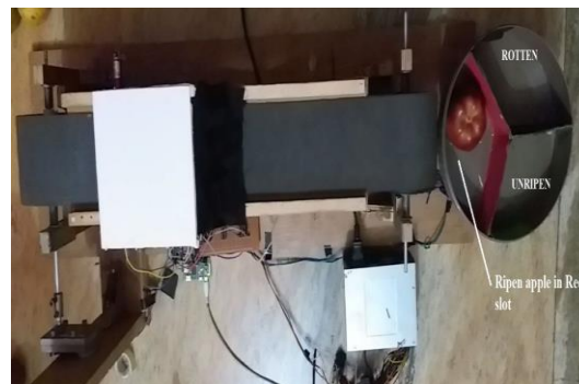
Figure 5.2 Detected ripen apple is collected in red slot.
