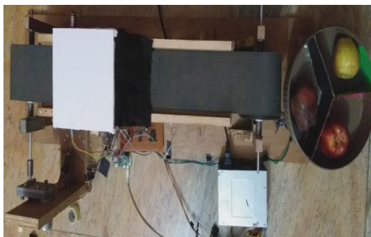
Figure 5.6 Detected rotten apple is collected in black slot.
