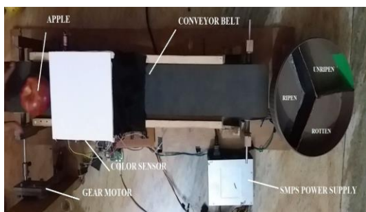
Figure 5.1 Placing the ripen apple on conveyor belt.
