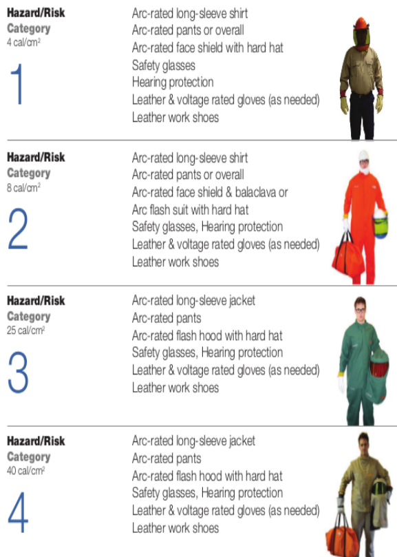
Figure 4: PPE levels and appropriate equipment [1]
